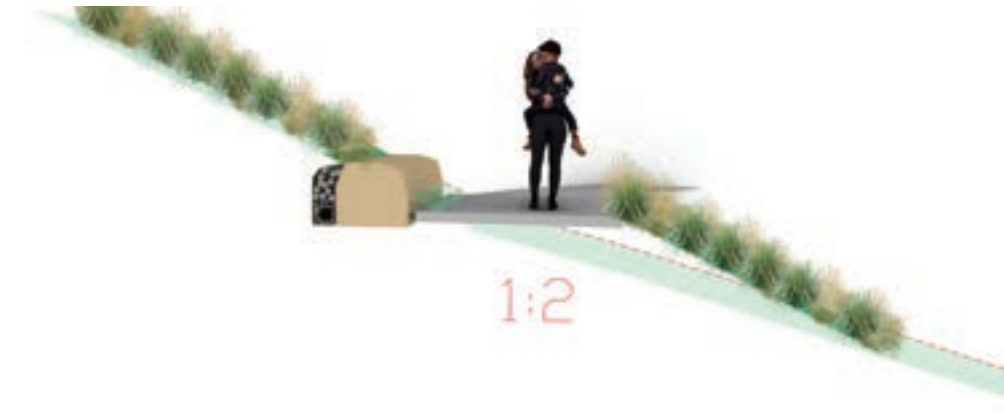
Figure 44, Above: Cut and fill with 1:2 batters and boulder edge at top of slope.
