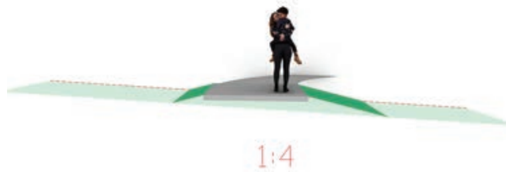
Figure 38, Above: Fill with 1:4 batters and swales.
