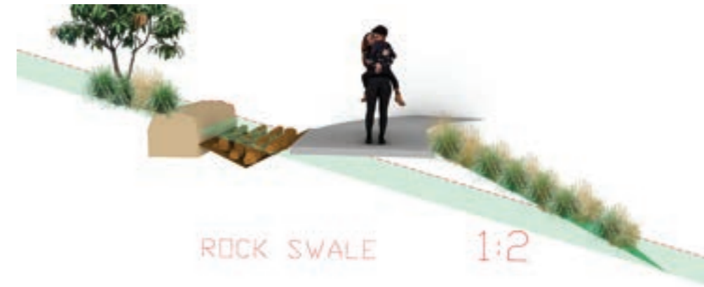
Figure 43: Cut and fill with 1:2 batter, rock swales with boulder edge at top of slope
