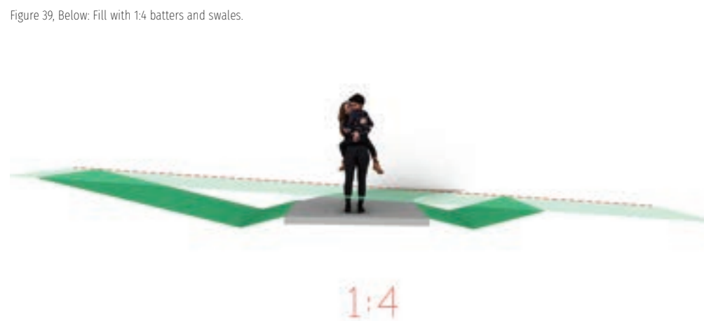
Figure 38, Above: Fill with 1:4 batters and swales.
