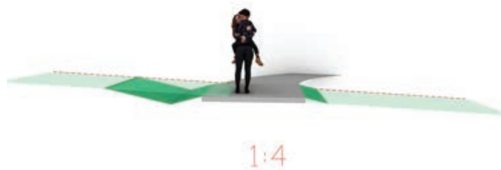
Figure 37: Cut and fill with 1:4 batters and swales.
