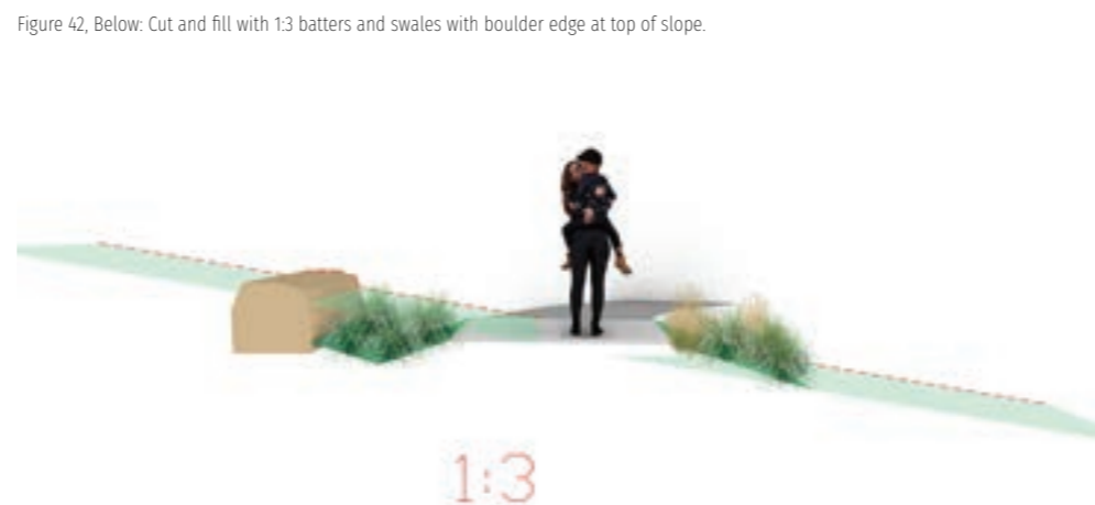
Figure 41: Cut and fill with 1:3 batters and swales.
