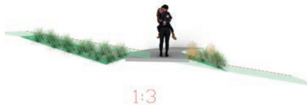
Figure 41: Cut and fill with 1:3 batters and swales.
